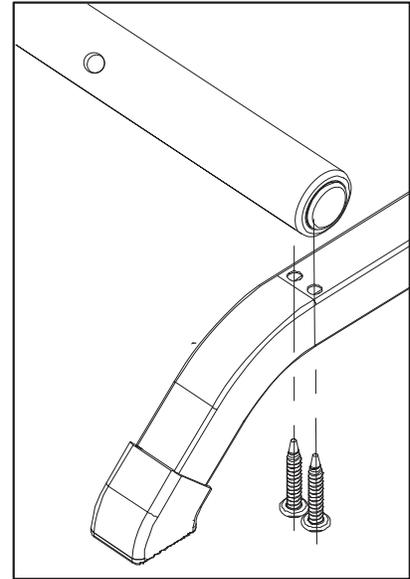
**3.** Level the bottom assembly on a flat surface.
