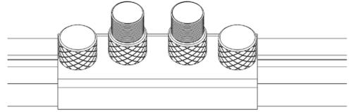
4. Depending on your desired mic/antenna position, screw the two security lugs into either the two inner or the two outer holes of the bracket and threaded insert.
