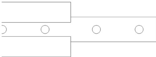
**1.** With the mic bar track facing up, slide the threaded insert into the end of one of the mic bars until two of the insert's holes are inside the bar, leaving the other two holes exposed.
