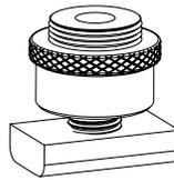
(4) multi-position mounting lugs with 5/8"-27 male threading
