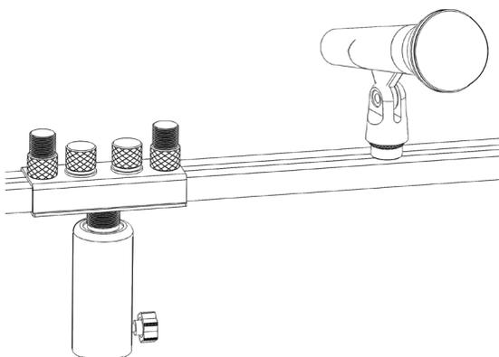
9. Mount mics (clips not included), antennas, or anything with a compatible 5/8"-27 threaded base to the six mounting lugs. Reference the weight capacity of the mic stand or speaker stand to avoid overloading.
