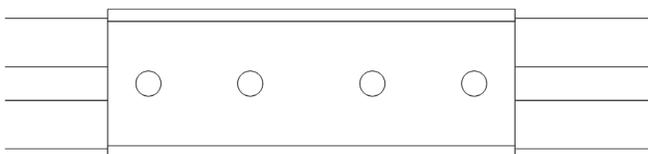
**3.** Slide the second mic bar into the opposite end of the center bracket so the threaded insert slides into the end of the mic bar as in step 1. Push the two mic bars together until they meet in the center. Align the four holes of the threaded insert with the four holes of the center bracket.
