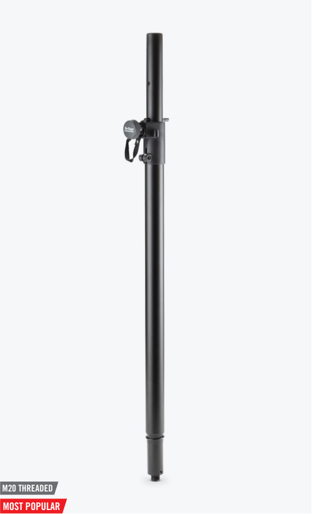
SUBWOOFER POLE WITH M20 THREAD SS7746 Length Adjustment: 30"–54" Speaker Pole Diameter: 1.375" Weight Capacity: 100 lb Construction: Steel Color: Black
