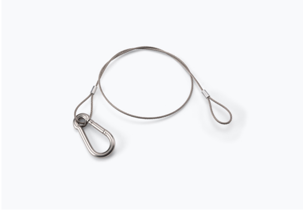
SAFETY CABLE SSACB28 Application: Backup attachment for overhead equipment Thickness: 3 mm Length: 28" Maximum Load: 60 lb Construction: Steel Includes: Carabiner
